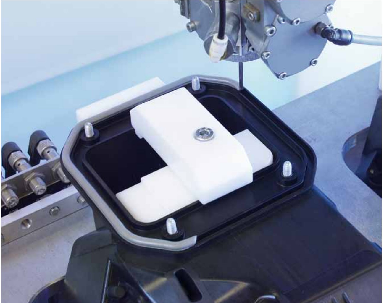
The CNC-controlled mixing head places the PUR gasket foam straight into the sealing groove of the moulded part.
