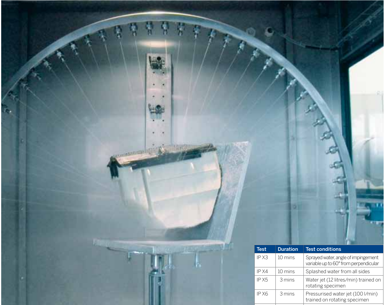
ECU box undergoing simulated rain test (IP X3 test in compliance with DIN 40050) in the ingress protection testing chamber.
